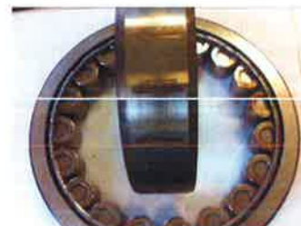
Figure 24: Surface marks (false brinelling)
