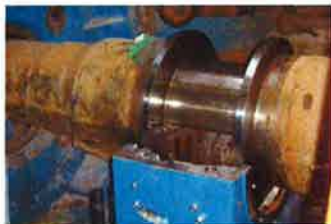
Figure 27: Corrosion on the shaft
