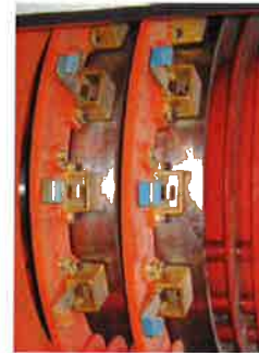
Figure 4: Brushes removed from the brush holder
