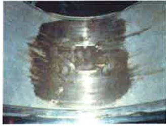
Figure 25: Marks on the bearing shell
